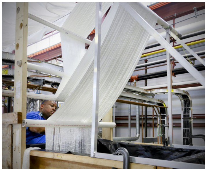
Figure 5.2. Production of lower-cost carbon fiber at the Carbon Fiber Technology Facility
